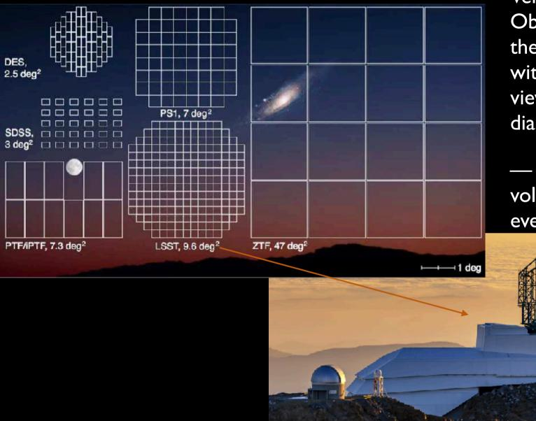
Vera Rubin Observatory will be the first telescope with a wide field of view and an 8m diameter mirror
